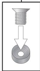
Screw through the locking washer to create the resting point for the end stop separator.
